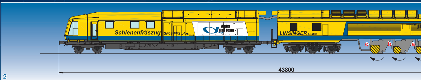
Reprofiling in a single pass with the two machines SF03-FFS (Fig. 1) and SF03-FFS plus (Fig. 2): milling, milling, finish grinding.
